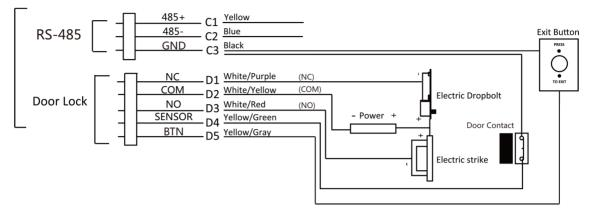
Figure 4-2 Device Wiring
