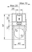
Right handed door shown in diagram Left handed door is the reverse SF\* = Passive leaf GF\* = Active leaf
