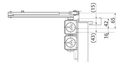
For mounting with drilling template acc. to EN 1154 Supplement 1 (fire and smoke protection doors) and for direct mounting.
