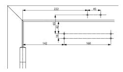
In compliance with EN 1154, Supplement 1, or for doors where direct mounting is not possible. Left handed shown in diagram Right handed is the reverse
