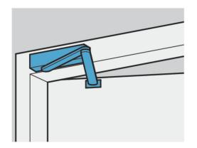
Closer on non-hinge side of door frame Right handed door shown in diagram Left handed door is the reverse
