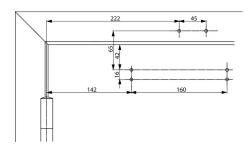
In compliance with EN 1154, Supplement 1, or for doors where direct mounting is not possible. Left handed shown in diagram
