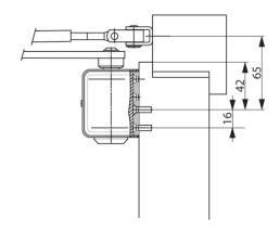
For mounting with drilling template acc. to EN 1154 Supplement 1 (fire and smoke protection doors) and for universal use
