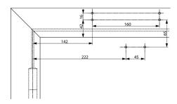
Closer on non-hinge side of door frame. For doors where direct mounting is not possible. Right handed door shown in diagram Left handed door is the reverse
