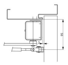
For frame mounting in case of deep jamb, headroom reduced by 70 mm. Check suitability for use on fire and smoke protection doors.
