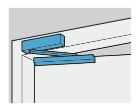
Closer on non-hinge side of door frame Right handed door shown in diagram Left handed door is the reverse
