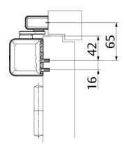
For mounting with drilling template acc. to EN 1154 Supplement 1 and for universal use
