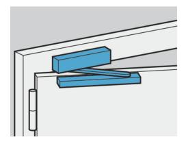
Closer on hinge side of door frame. Left handed shown in diagram Right handed is the reverse
