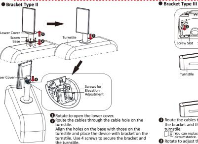
1 Route the cables through the cable hole on the turnstile. Align the holes on the bracket and those on the turnstile and place the bracket on the You can replace the decoration sheet by the arch shaped decoration for some
